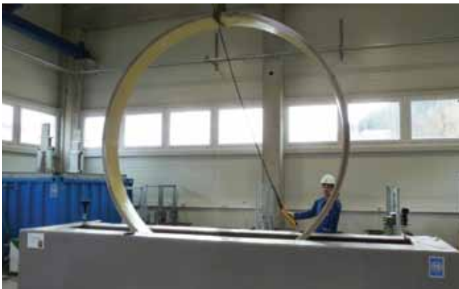
Above: Abrasion resistance test. Below: Long-term ring stiffness test.
