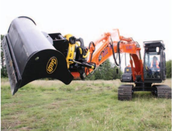
Hitachi excavator with Engcon attachment
