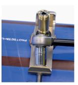
3. Ensure pre-cutter is installed, and replace outlet banjo with large seal top and bottom.
