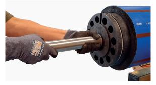
1. First mark the required length of pipe to be scraped (see table on page 11). Ensure that the correct size collet for the pipe to be scraped is fitted to the mandrel. Adjust the collet by twisting the mandrel shaft anti-clockwise until it achieves its smallest outside diameter. Slide the collet into the bore of the pipe, allowing 20mm of pipe to show after the collet, to allow for the barrelling effect found at the end of the pipe.
