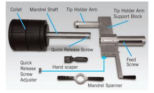
For Protecta-Line sizes above 180mm, the surprep scraper is a dedicated tool for each pipe size, with the cutter set to produce the required outside diameter. Adjustments must be carried out by a competent person and can only be done on site as each pipe batch requires repeated scraper calibration.
