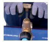
Retract the cutter until it seals fully against the inside top of the body.
