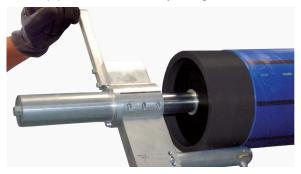
6. When the required length of pipe has been prepared, raise the quick release screw to its top position (about one and a half turns). The quick release screw can be accessed through the slot in the feed screw housing tube.
