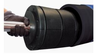
9. Remove the collet and mandrel from the pipe. The collet should be removed to a clean dry and safe area. If there are any areas of pipe that have not been prepared properly, then the hand scraper should be used to complete the preparation process.
