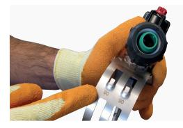
2. Unhitch the lower part of the ferrule understrap from the tabs on the upper part of the strap. Leaving the bolt in place, fit the ferrule squarely around the main, re-attach the understrap to the appropriate tabs.
