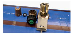
Unscrew body top and outlet banjo ensuring all seals are retained and set aside, which is only applicable on mains 200mm and above. Ensure that the sealing O-ring is in place under the upper ferrule strap (take care not to damage this on the protruding sleeve).
