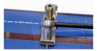
Fit strap squarely on main and tighten bolts to a torque 20Nm - 24Nm. Make sure both bolts are tightened evenly.
