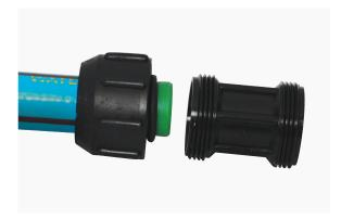
4. Offer the body of the fitting to the Protecta-Line pipe end and screw the nut on to the fitting body. Continue to tighten the nut until the thread on the body is no longer visible.
