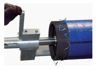
5. Taking care to avoid damaging the quick release nut and feed screw, rotate the tool in a clockwise direction with a slight force pushing forward. Once the feed screw has engaged with the quick release nut, it will now proceed to travel along the length of the mandrel shaft, removing the outer barrier layers and preparing the pipe for electrofusion jointing.
