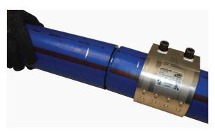
5. Ensure the shells are flush with the pipe ends or for the straight coupler, centre the shell between the depth penetration marks. The fitting is ready to be tightened. Set the torque wrench to the value indicated on the label of the shell.
