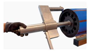
4. Ensure that the tip holder arm has been located in the hole corresponding to the pipe size in the tip holder support block. Locate the tool onto the mandrel shaft taking care not to damage the bore of the tool. Slowly slide the tool along the mandrel shaft using a twisting action, until the feed screw touches the quick release feed screw nut.
