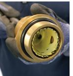
**3.** Ensure the ball valve is in the fully open position. Fit the drill head to the outlet of the ferrule.
