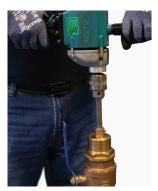
5. Disconnect power supply and remove drill from stem. Withdraw stem, until the cutter is fully returned into the drill head and fully close the valve (handle is horizontal to valve) before removing the drill head from the outlet of the ferrule.
