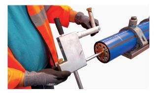
6. Slide the body of the Protecta-Line surprep scraper onto the mandrel, depress the release button and position the cutter close to the edge of the pipe.
