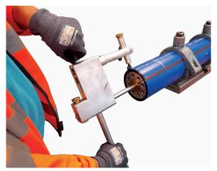
**9.** Rotate the knob on top of the post through 90° so that spring pressure is applied to the cutter.
