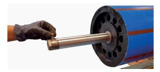
**3.** Once the mandrel is secure and is parallel with the pipe bore, screw down the quick release screw to its full extent (about one and a half turns) using the adjuster, which is stored at the base of the tip arm support block.
