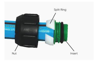
**3.** Slide the split ring along the Protecta-Line pipe until it is up against the insert. Snap the nut over the split ring.
