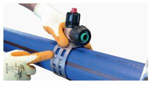
**3.** Tighten the strap bolt with a 13mm socket wrench or spanner to 12–14Nm of torque.
