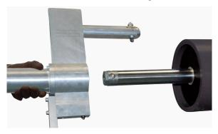
7. The tool can now be removed from the mandrel shaft.
