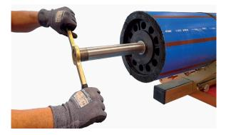
2. Adjust the collet by twisting the mandrel shaft clockwise until the mandrel becomes secure in the bore of the pipe and tighten with the mandrel spanner. To achieve the correct alignment parallel to the pipe bore, a joggling action in all directions is required. The collet also acts to re-round the pipe so check for gaps between the collet and the bore of the pipe.
