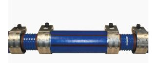
7. Tighten the hex socket head bolts until the set torque is achieved in each bolt. The pipe will relax after the set torque is achieved, so after a minute or more, retighten the bolts to the set torque. Repeat until less than a quarter turn is needed to reach the set torque.\*
