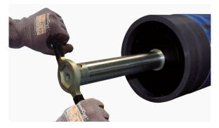
**8.** Loosen the collet using the mandrel spanner on the mandrel shaft in an anti-clockwise direction until free.
