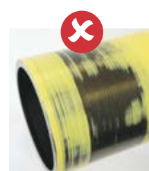
Incorrect pipe preparation for electrofusion
