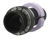
The corrugated pipe seal WRD is the optimum sealing solution for corrugated cable ducts. The patented ring clips ensure a uniform distribution of the contact pressure and gentle sealing without any penetration of the sealing rubber into the pipe corrugation. This prevents deformation of and damage to the corrugated pipe in the first place.
