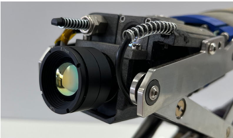
High definition thermal image sensor locates leakages
