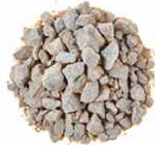
TYPE 3 SUB-BASE OPEN GRADED SHW CLAUSE 805
