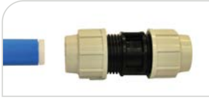
Insert liner into pipe (metric 20mm-63mm only) and slacken nut until half the thread is visible.
