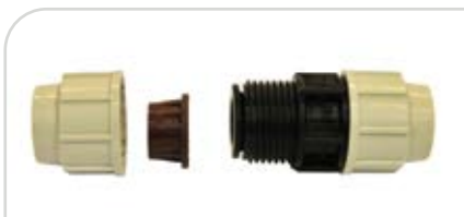
Remove nut from fitting and discard white split ring (except 35, 42, and 54mm copper, where the white split ring is used as a spacer). Push black rubber seal into fitting body and assemble components in the order shown above.
