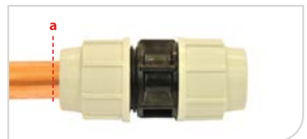
Push and twist the pipe through the nut, adaptor and metal ring into the body of the fitting, until the mark is in line with the end of the nut as shown. Tighten the nut with a PLASSON wrench.
