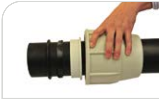
Draw the nut, collars, and 'O' ring over the end of the pipe to a distance of approx. 250mm (put the white split ring to one side for later use).
