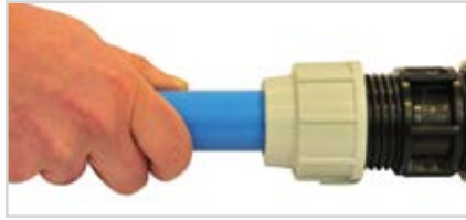
Push pipe into body, through the nut, split ring, and 'O' ring.
