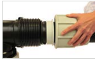
Insert the pipe into the body of the fitting until it meets the interior stop. Then draw the 'O' ring and collars close to the body of the fitting.
