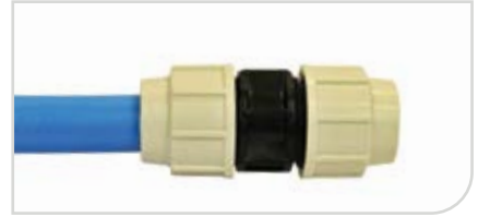
Tighten nut firmly: Hand tight on pipe 20mm (1/2") - 32mm (1"), on pipe 40mm (1 1/4") and above use a PLASSON wrench.
