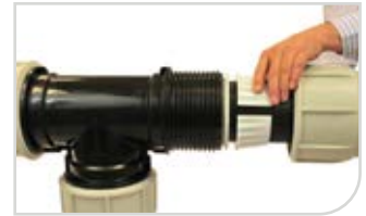
Open the white split ring and mount onto pipe with larger side against the collar ensuring that both parts meet the body of the fitting. Screw the nut tightly onto the fitting using a PLASSON wrench.
