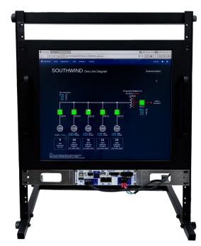
The OrionSX is ideal as a distributed HMI server, easily mounted with a monitor in multiple locations in large transmission substations. The OrionSX browser can be pointed to the substation RTU to view the same pages; no points configuration or page configuration required.
