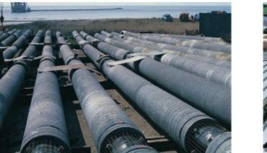
Subsea joints of sea-outfall, Atlantic Ocean, protected with Densopol™ Marine Tape System.
