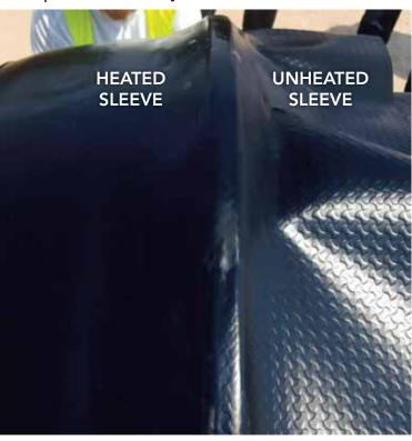
Available in several grades, tested to meet the requirements of DIN EN 12068, Premier Shrink Sleeves<sup>™</sup> are cost effective and easy to install with the help of a thermal indicator which aids correct application every time.
