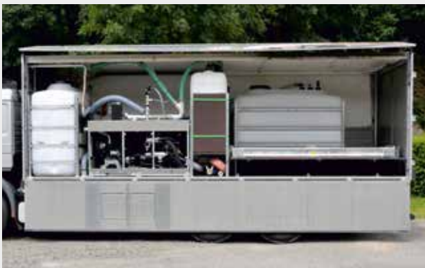
Everything is on board: truck platform for mixing systems, drive and accessories.
