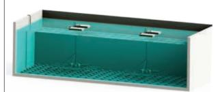
Due to malfunctioning existing aeration equipment, Mapal floating units were installed without removing the existing diffusers, providing supplemental oxygen to the reactor.
