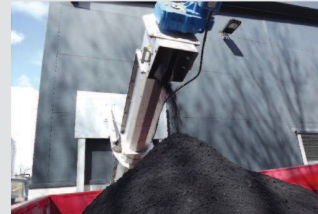
De-watered sludge cake
