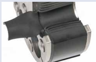
Standard seals with segmented ring technology for individual adjustment to cable diameters on site.
