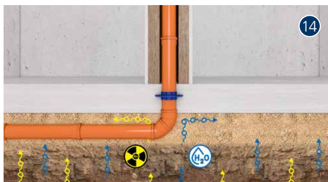
KGF110 set in concrete
