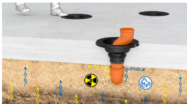
AT110 with drain pipe installed
