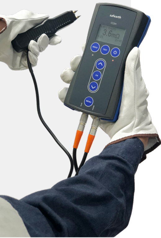
Continuity testing using the Safearth CS3 Site Continuity Meter
