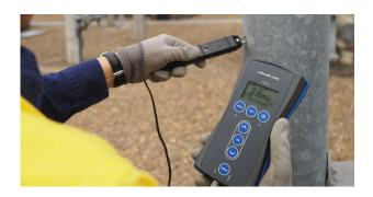
The use of a comparably low 1A test current in the CS3 enabled this serious defect to be identified accurately without causing any negative impacts, whereas a high current test (10A or greater) may have caused damage to the control wiring, likely resulting in an outage.
