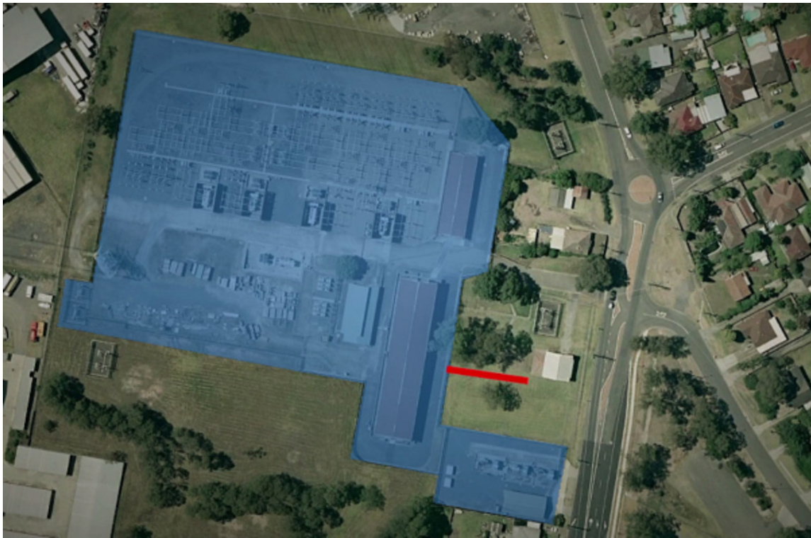
An example of a poorly executed three-point test
