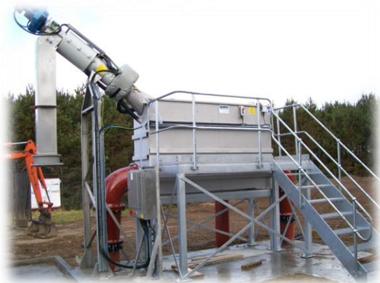
Tank mounted screen with access platform
