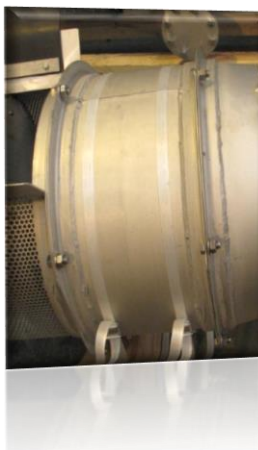
Intermediate shell bearing to prevent damage to auger and basket
