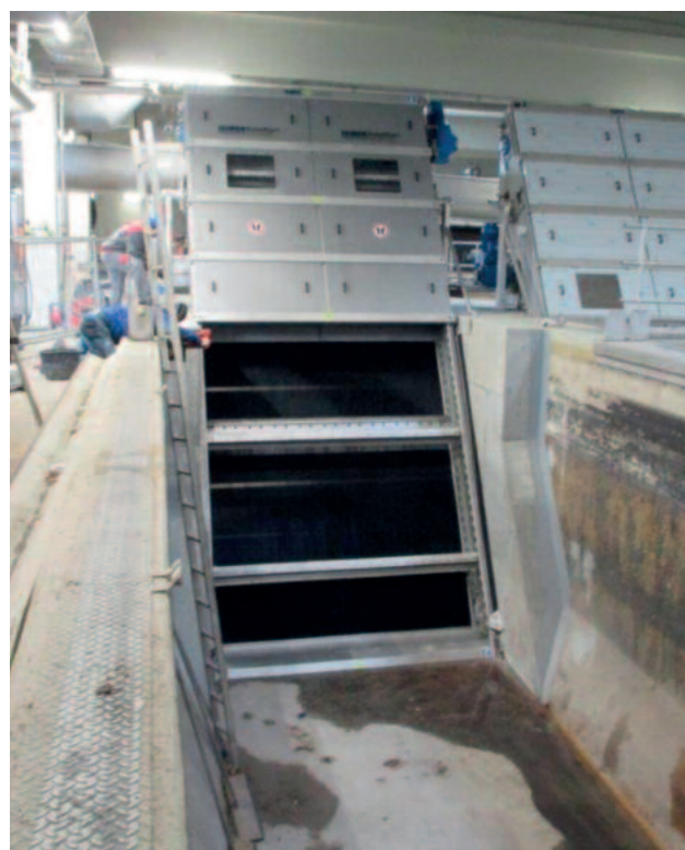
Multi-Rake Bar Screen RakeMax® Hybrid as fine screen with a machine width of 3.2 m
