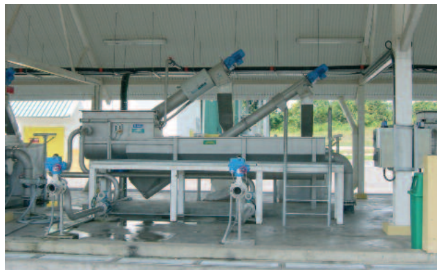
HUBER Sludge Acceptance Plant ROTAMAT® Ro3.3 with unaerated grit trap and integrated grit classifying screw
