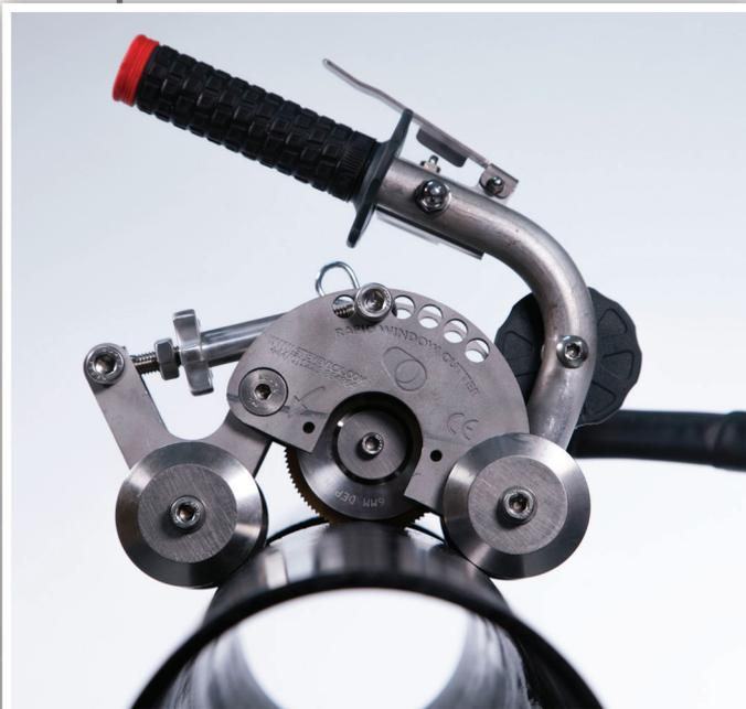
The Rapid Window Cutter for Steel mains
