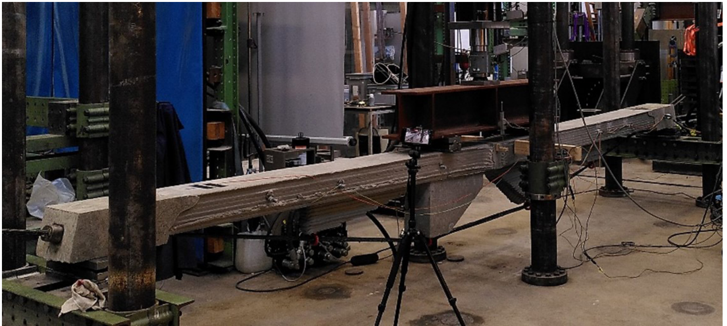
Fig. 9: Test set-up for 6m long DTU test beams of type MM-01
