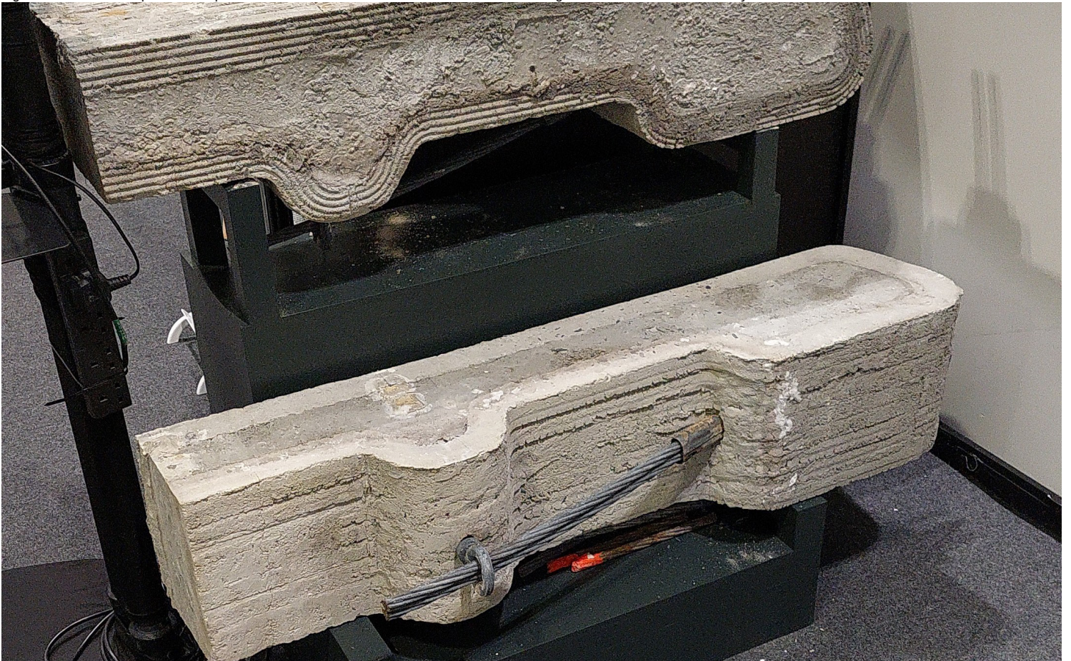
Fig. 8: Example MM-02 beam after 132 mins at 1100 deg. C - minimal signs of damage
