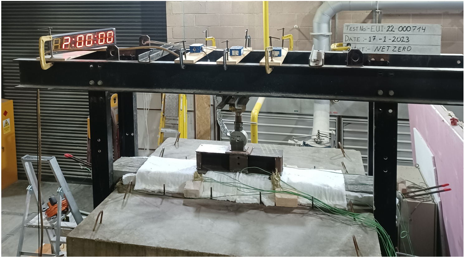
Fig. 10: Fire test set-up at Efectis, Belfast, showing full integrity at 2hrs fire duration
