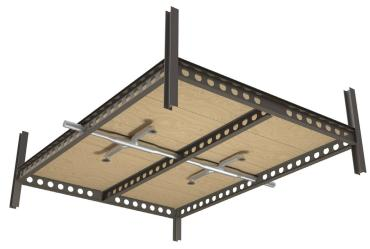
GreenBox is a climate-friendly floor cassette system that performs like a concrete floor, but with less mass and a fraction of the embodied carbon. The design combines a stiff timber structure with a proprietary filling that dampens vibration and improves acoustic and fire performance. And installation is simple: just lift in prefabricated cassettes and connect with screws – no special skills or equipment are needed.
