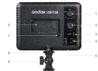
(1) Select Dial for Color Temperature (2) Select Dial for Light Brightness (3) Battery Indicator Button (4) ON/OFF Power Switch (5) Heat Dissipation Hole (6) Lithium Battery Compartment (7) Battery Unlock Button (8) 1/4" Bracket Mounting Hole (9) L-type Bracket
