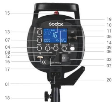
(1)AC Power Socket (2)Sync Cord Jack (3)Power Switch (4)Modeling Lamp Output Controller (5)Flash Output Controller (6)Modeling Lamp Button (7)GR/CH Button (8)Slave Model Button (9)Test Button (10)Digital Display (11)Modeling Lamp Indicator (12)Buzz Button (13) Custom Function Button (14)Test Indicator Lamp (15)Light Sensor (16) Wireless Control Port (17)Fuse (18)Mounting Bracket (19)Umbrellas Input (20)Direction Adjusting Handle
