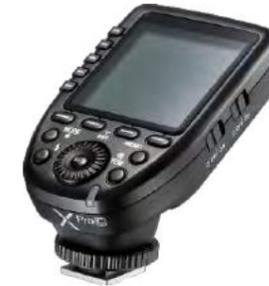
Xpro Series TTL Wireless Flash Trigger can not only control the flashes with built-in Godox wireless X system e.g. camera flashes, outdoor flashes and studio flashes, but also can control the flashes without Godox X system by 2.5mm sync cord jack. XProC/XProN/XProS/XProF/XProO/XProP separately applies to Canon, Nikon, Sony, FUJIFILM, Olympus/Panasonic and Pentax series cameras.
