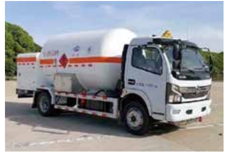
LPG tank lorry with pump
