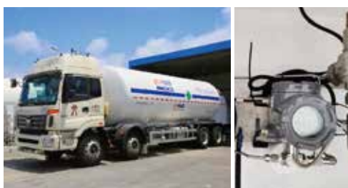
Intelligent Telemetry Terminal (Lorry Tanker Type)
