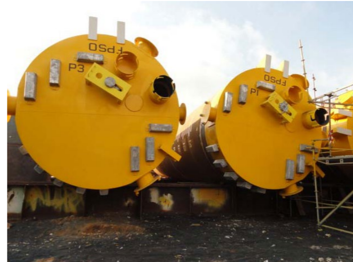
12 piles fabricated making a Total: 700 mt / 17m x 4m Ø each
