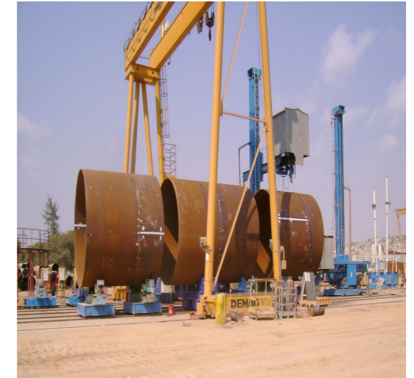
12 piles fabricated making a Total: 700 mt / 17m x 4m Ø each
