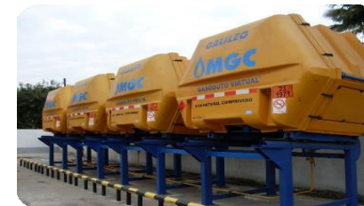
Compressed Natural Gas (CNG) Virtual Pipe Line
