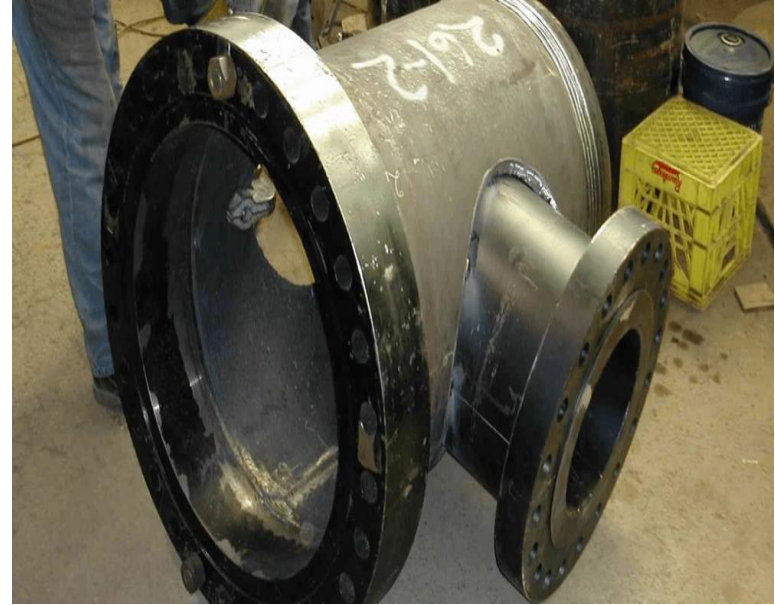
Fit-up of Nozzle to Vessel Shell
