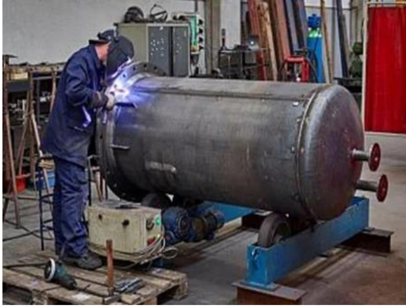
Welding of Flanges to Boot Shell
