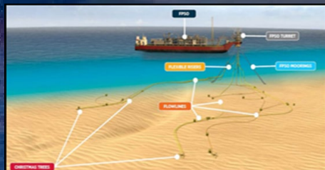
Development Concept (Drilling Rig + FPSO)
