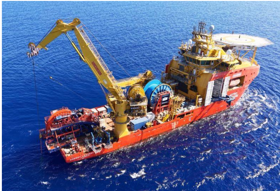
TCP installation Reel, Reel Drive System, tensioner and chute on deck
