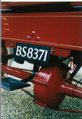
The rear axle is almost totally enclosed.
