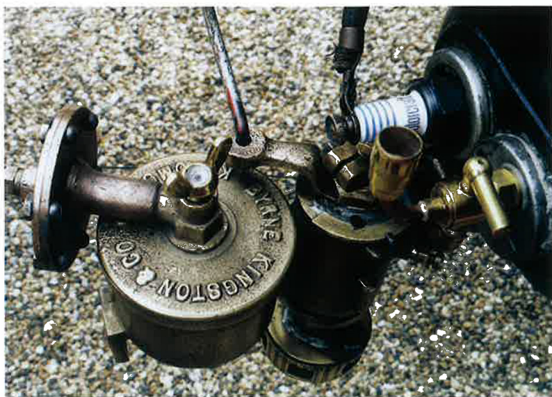
above: On this early Model 'A', the carburettor is made by Byrne Kingston and Co, Kokomo.
