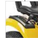
**MECHANICALLY SUPPORTED CUTTING HEIGHT ADJUSTMENT**
