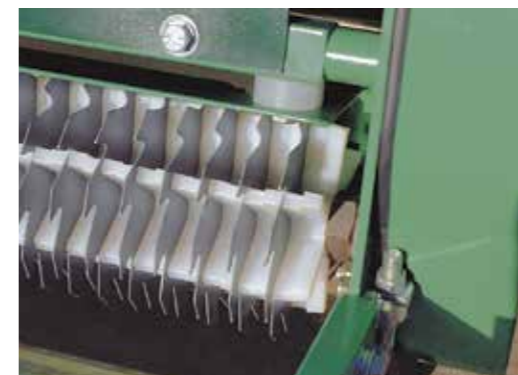
Tungsten tipped blades and finned spacers for ultimate cutting and collection performance.
