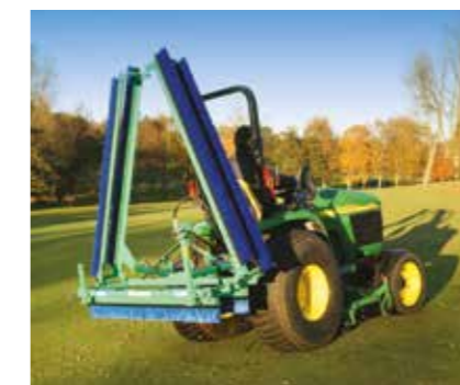
Hydraulic Maxi-Brush folds up without leaving your seat.
