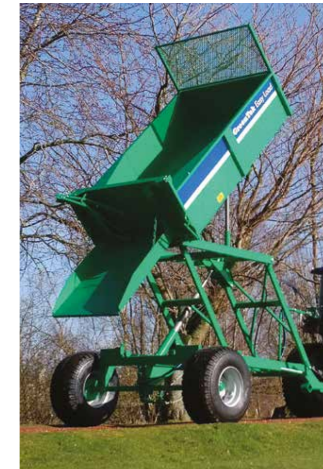
Wheels spaced outside body width provide extra stability for high tipping.
