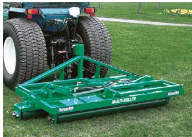
The three rollers can be used in-line for intensive rolling
