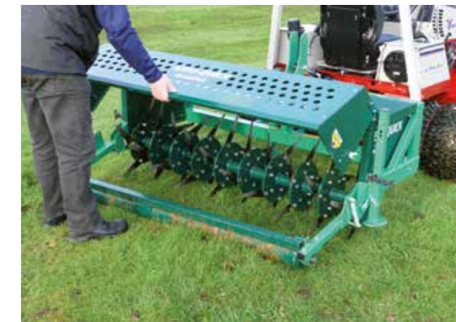
Hinged rear guard for easy access to changeover attachments
