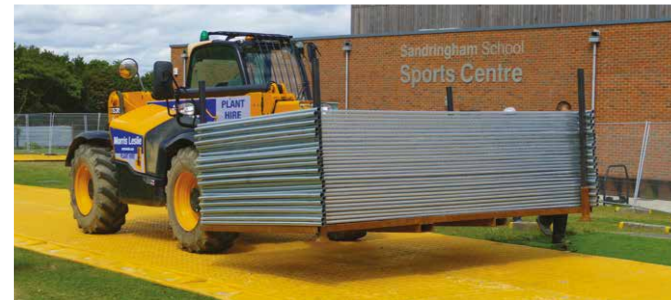
XtremeMat: Create access roads for heavy plant
