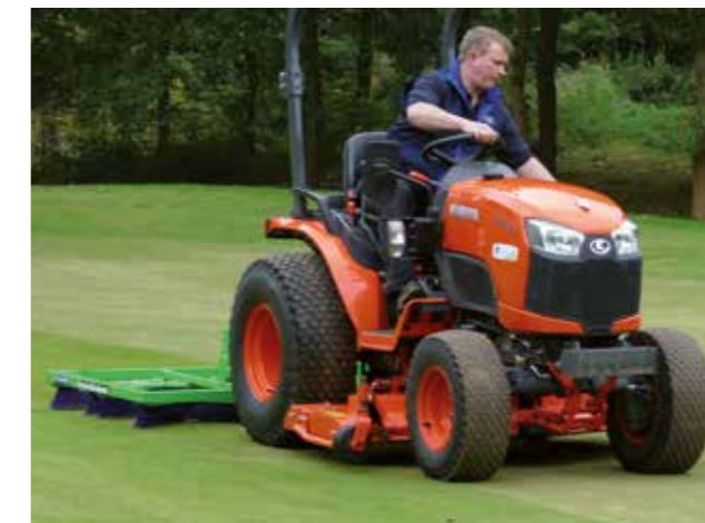
Brushes sand down coring holes
