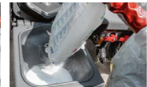
The high intake capacity of the induction hopper ensures short downtimes and high daily output.
