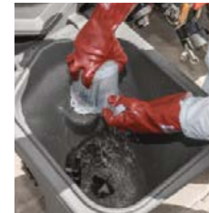
The lowerable induction hopper for ergonomic operation and easy filling.
