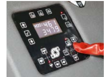
Using AutoFill, the tank can be automatically filled up to the required volume.
