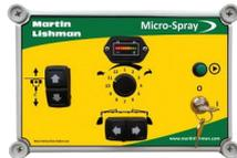
*3-section valve block with pressure regulation and agitation supplies the 2.5m or 3.5m boom. Spray application rates, pump pressure, bout marker selection and a battery level indicator can be accurately and quickly controlled or viewed by the operator.*
