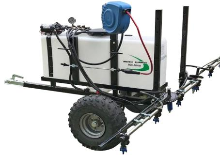
*Mini-Spray Trailed 125 litre with 2.5m 6-nozzle 3-section folding boom and retracting hose reel with hand lance*
