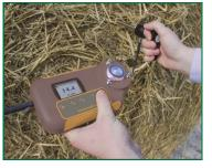
Bale Temperature Probe 600mm probe for checking hay and straw bale temperatures
