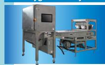
The machine body is a dividable structure for easy cleaning and maintenance. Belt conveyor is easy to remove.
