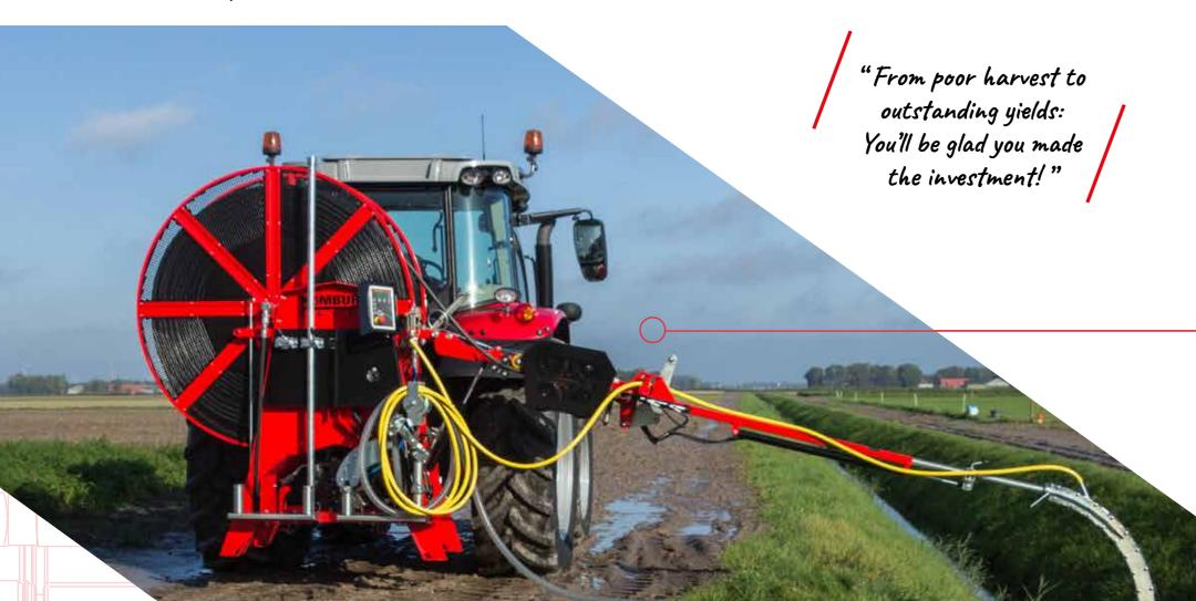
The Delta offers more ease of use as a draincleaner than the Blizz. This is the ideal machine for anyone who maintains drainage systems on a frequent basis and needs to cover a large area. This is because it offers hydraulically operated height adjustment, extension, retraction and folding of the drainage arm and length adjustment of the guide arm.
