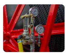
Both pressureguages for water and hydraulics are easy to check.
