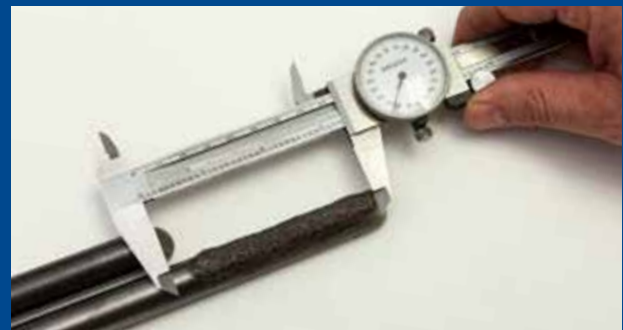
10,000 ACRES OF WEAR COMPARING A MAX LIFE TINE TO A REGULAR TINE.
