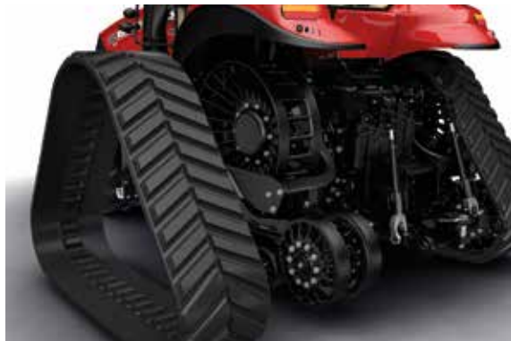
The positive drive system eliminates slippage between the drive wheel and rubber track in all conditions.
