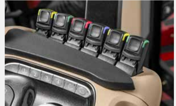
Configurable control switches with changing colours allow individual assignment of the rear control units
