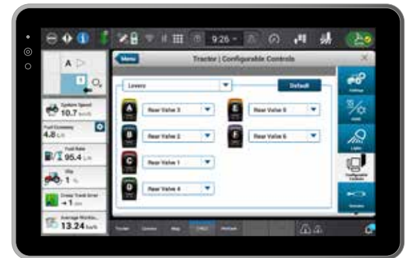
Shortcut keys bring you directly to the settings menu to configure your remote valves.
