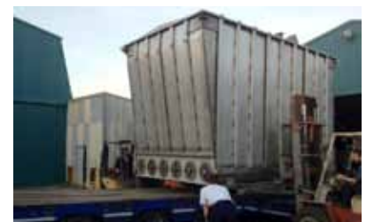
Stainless Steel intake hopper with 6 no. 400mm diameter screws
