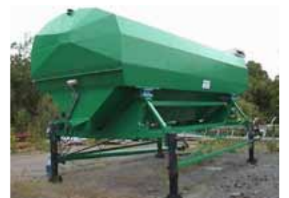
Vertical Lime / Cement 40 tonne Silo
