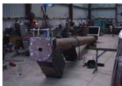
Special Screws 500mm \phi , 18 mtrs long
