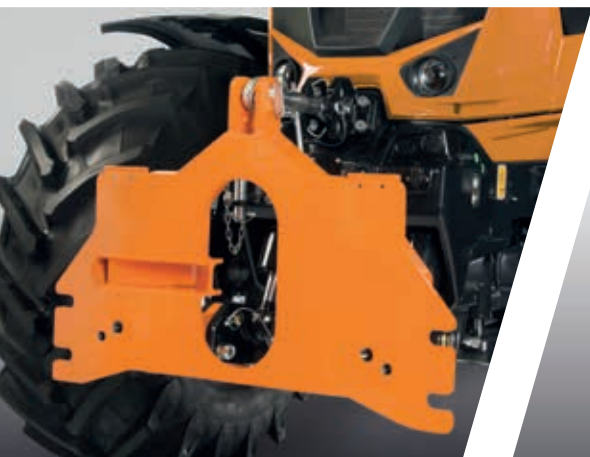
> Sauter municipal mounting (category 3/5). For fast and robust mounting of special equipment.
