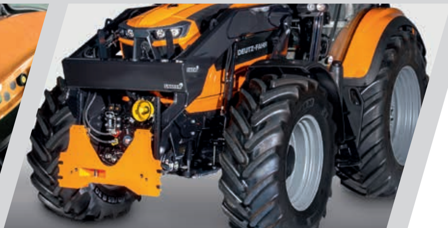
> Support frame from Sauter with adjustable communal pallet (category 3/5) and axle support for heavy attachment loads and outrigger.
