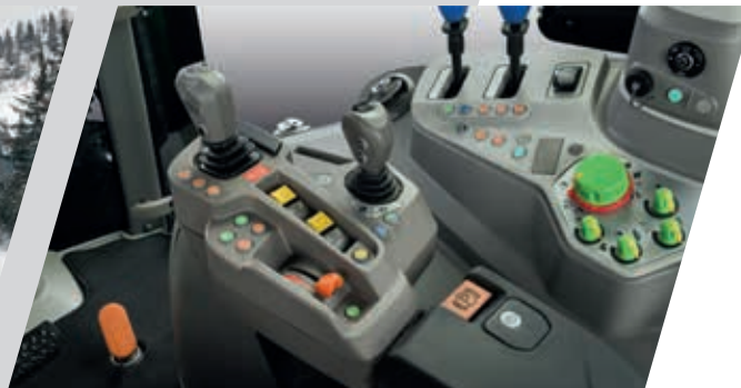
> MaxiVision* cab with mixed rear hydraulic spool valves and electronic front loader control.
