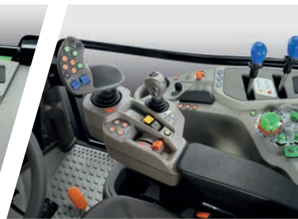
> TTV satellite armrest with MaxCom joystick.
