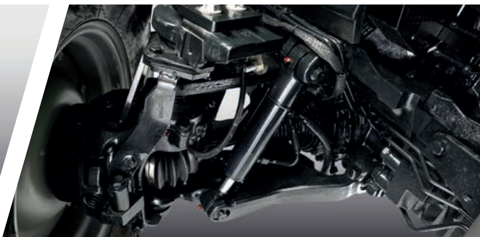
> Independent front axle suspension.
