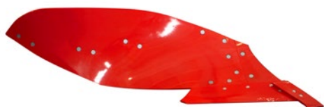
MP4WD - Full-mouldboard, semi-helical, ideal for heavy/wet soils for tractors with wide wheels ( \leq 800 mm). (Working depth 15-30 cm).
