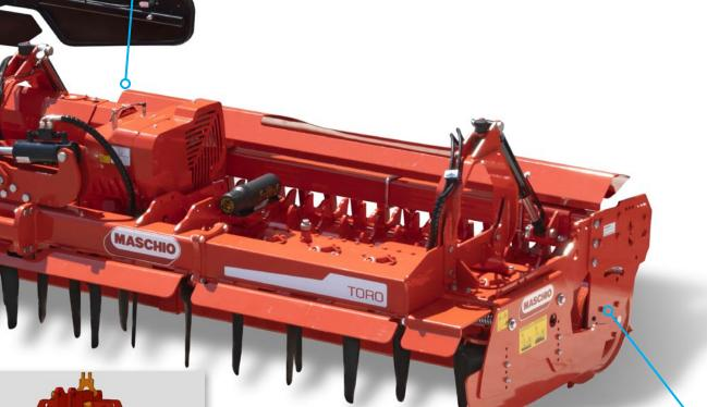
Air-cooling device for oil gearbox
