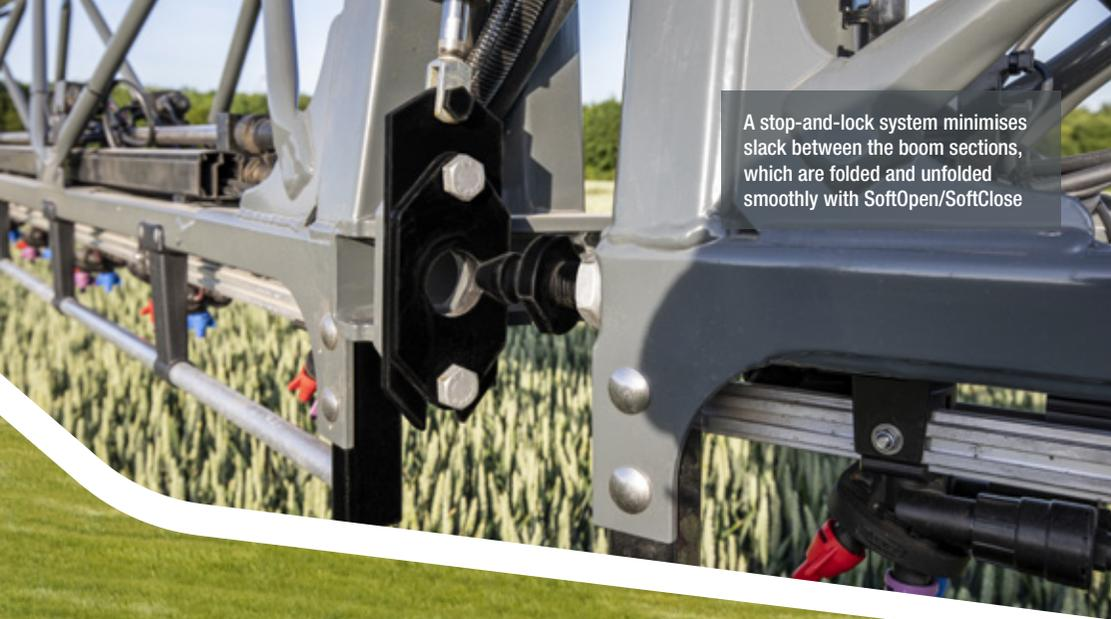
A stop-and-lock system minimises slack between the boom sections, which are folded and unfolded smoothly with SoftOpen/SoftClose
