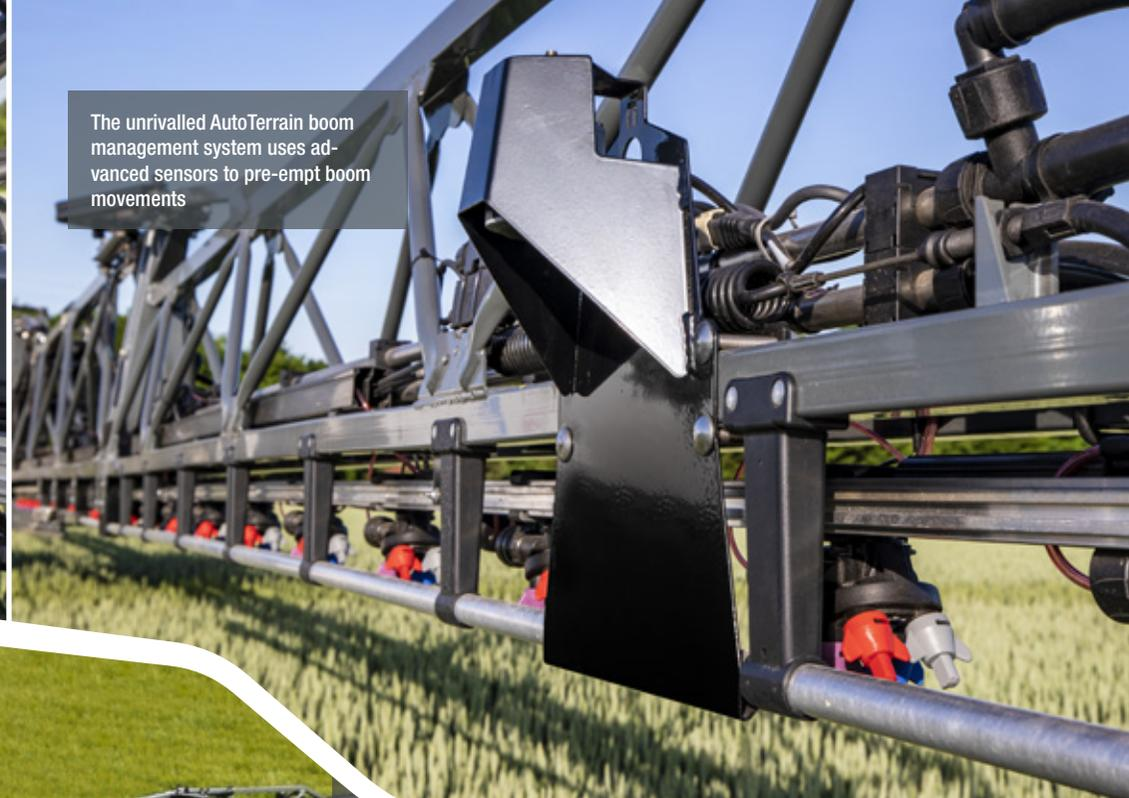
The unrivalled AutoTerrain boom management system uses advanced sensors to pre-empt boom movements
