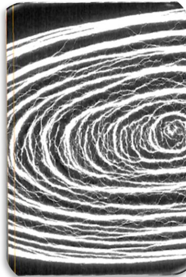
Cross-sectional structure of an extruded soy protein fibre by X-ray tomography
