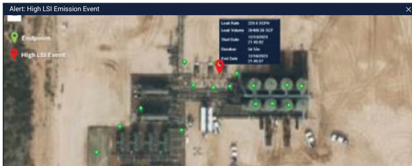
MethaneTrack™ LSI alert displaying emission duration, rate, location and volume.
