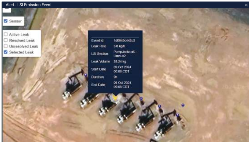
Emission details on MethaneTrack™ platform specifying location, volume, and duration of leak
